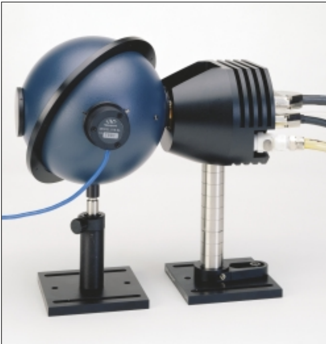
Figure 15. Close-up view of the calibrated 6 inch diameter integrating sphere and silicon detector assembly (Model 819S-06-SL-CM-DV) and water cooled laser diode mount (Model 762W-xx-TE) used in the laser diode experimental setup of Figure 14. This laser diode mount has a built-in TEC.
