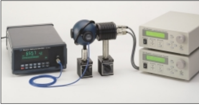
Figure 10. Test setup for output light power measurement of a laser diode with output power of up to about 3 Watts.
