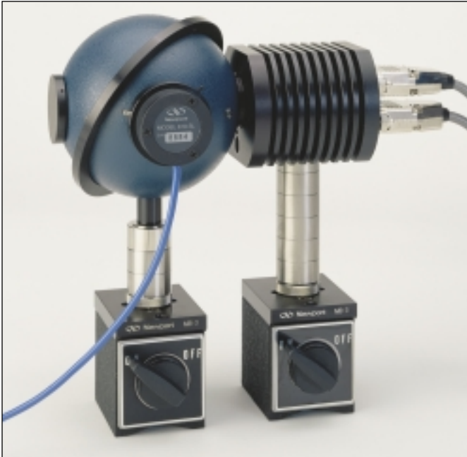
Figure 11. Close-up view of the calibrated 4 inch diameter integrating sphere and silicon detector assembly (Model 819S-04-SL-CM-DV) and laser diode mount (Model 760) used in the laser diode experimental setup of Figure 10.
