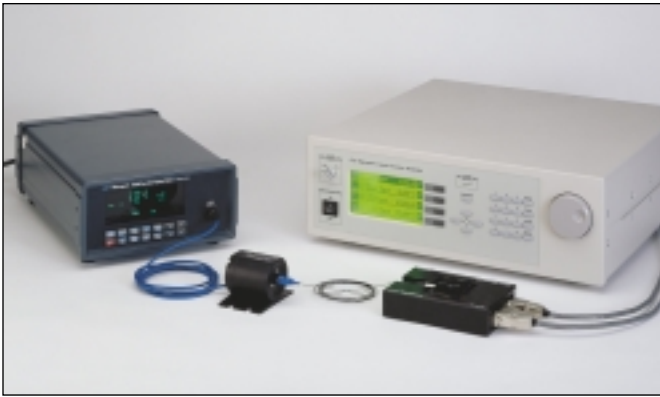
Figure 17. The experimental setup used to measure the output light power of a fiber pigtailed telecom laser diode. A small size diameter integrating sphere, Model 818-IS-1 Universal Fiber Optic Detector is shown with a 744-TEC Series Telecom Laser Diode Mount and Model 8008 Modular Laser Diode Controller.
