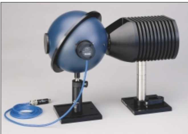
Figure 8. A 6 inch diameter 819S integrating sphere equipped with an 818-SL detector. The laser is mounted on Newport's Model 762 air cooled high-power laser diode mount. This assembly is used for optical power measurements of a CW high-power laser diode bar.
